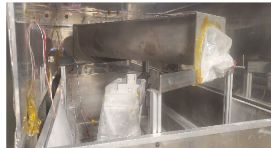
Fig. 2. Screw and Piston Conveyors in DTVC.
